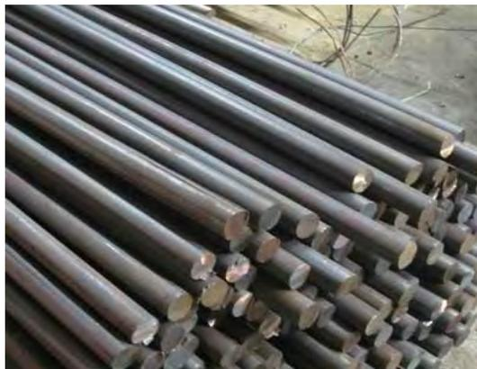
The round bars are made by rolling of billets into the required round sizes. We get the round bars manufacture on job work basis from third party manufacturers. Our company provides requisite billets for getting round bars manufacture on job work basis from third party manufacturers.
