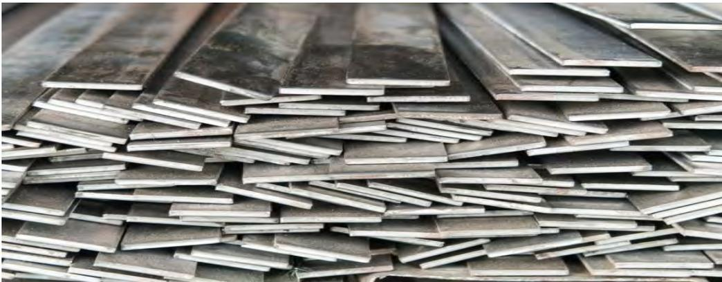
The SS Flat bars are supplied to customers in various thickness from 10.5 mm to 21 mm. The SS Flat bars are made by re-heating the billets and rolling into required size.
